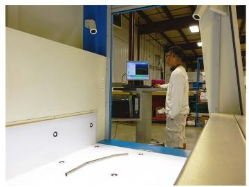
Globe Engineering Co. Inc. invested in two optical measurement systems, TubeInspect models P8 and P16. The smaller unit measures tube up to 39 in. long in diameters from 0.040 to 5 in. The tolerance is  $\pm$  0.001 in. The larger unit handles tube up to 102 in. long in diameters from 0.12 to 8 in. long. The tolerance is  $\pm$  0.003 in.
